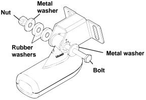
Assemble transducer and bracket.
